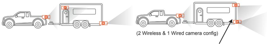
Having two cameras at the back, one camera can be optimised for parking (top down view) whilst the other can look backwards and be used as a rear-view mirror substitute.
