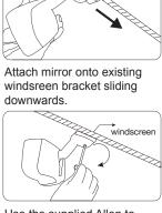
Use the supplied Allen to tighten fixing screw.
