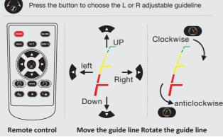
Guide lines are designed to assist with parking and judging distances, but should not be relied on solely when reversing.
